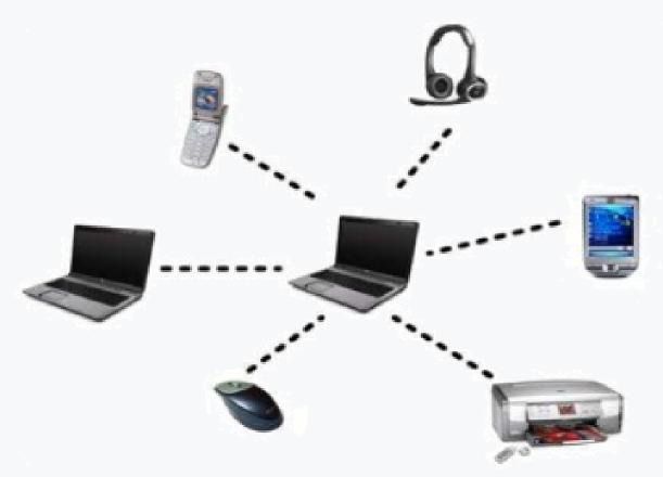
PAN networks are designed to serve a single user or a small group of devices, making them highly efficient for short-range communication. Examples include connecting a smartphone to a Bluetooth speaker or sharing files between a laptop and a tablet. Though limited in scope, PANs are an essential part of everyday technology usage.
