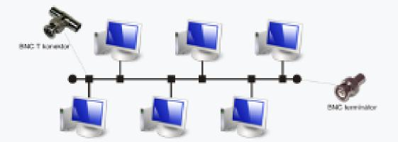
Devices in a bus topology take turns sending data on the shared medium, which helps keep costs low by minimizing cabling. However, as more devices join the network, the likelihood of data collisions increases, leading to slower performance. Bus topologies are also less reliable, as a failure in the central cable means that communication across the entire network is disrupted.
