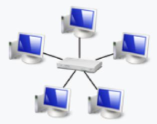
Since all communication passes through the central node, this topology provides excellent control over the flow of data. Additionally, troubleshooting is simpler because a failure in one device doesn't affect the entire network. However, the dependence on a central node means that if this node fails, it can lead to a complete network outage, making redundancy mechanisms important for critical applications.
