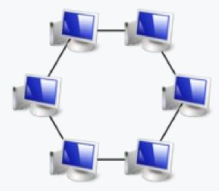
In ring topology, data moves in one direction (unidirectional) or two directions (bidirectional), depending on the setup. If a device fails or a connection breaks, the entire network can be affected unless there's a backup mechanism in place, such as a dual-ring configuration. Ring networks can be useful in smaller environments, but their vulnerability to individual points of failure makes them less desirable in larger systems.
