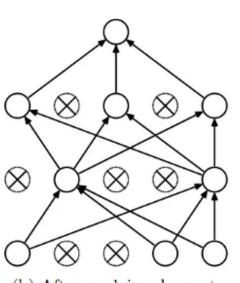
(b) After applying dropout.
