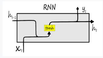
As can be seen in the previous image the non-linear activation function is applied to get new state  $h_t$  and the output  $y_t$ .
