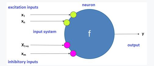
The logic neuron system contains excitatory inputs (binary variables  $x_1, x_2, ..., x_n$ , which **amplify the response**) and inhibitory inputs (binary variables  $x_{n+1}, x_{n+2}, ..., x_m$ , which **weaken the response**).
