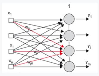
In the course of active dynamics, the network generally realizes the display from  $\mathbf{R}^n \rightarrow \mathbf{R}^m$ , which was set during the adaptation dynamics. The specific values of the output values are given by the activation transfer functions of the output neurons, that is, for example, in the case of sigmoidal activation functions approximating a sharp nonlinearity, it is the realization of the display from  $\mathbf{R}^n \rightarrow (\mathbf{0}, \mathbf{1})^m$
