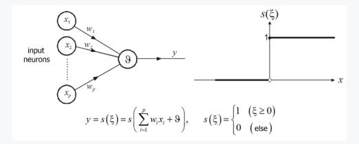
Weight coefficients and threshold coefficient are real variable parameters
